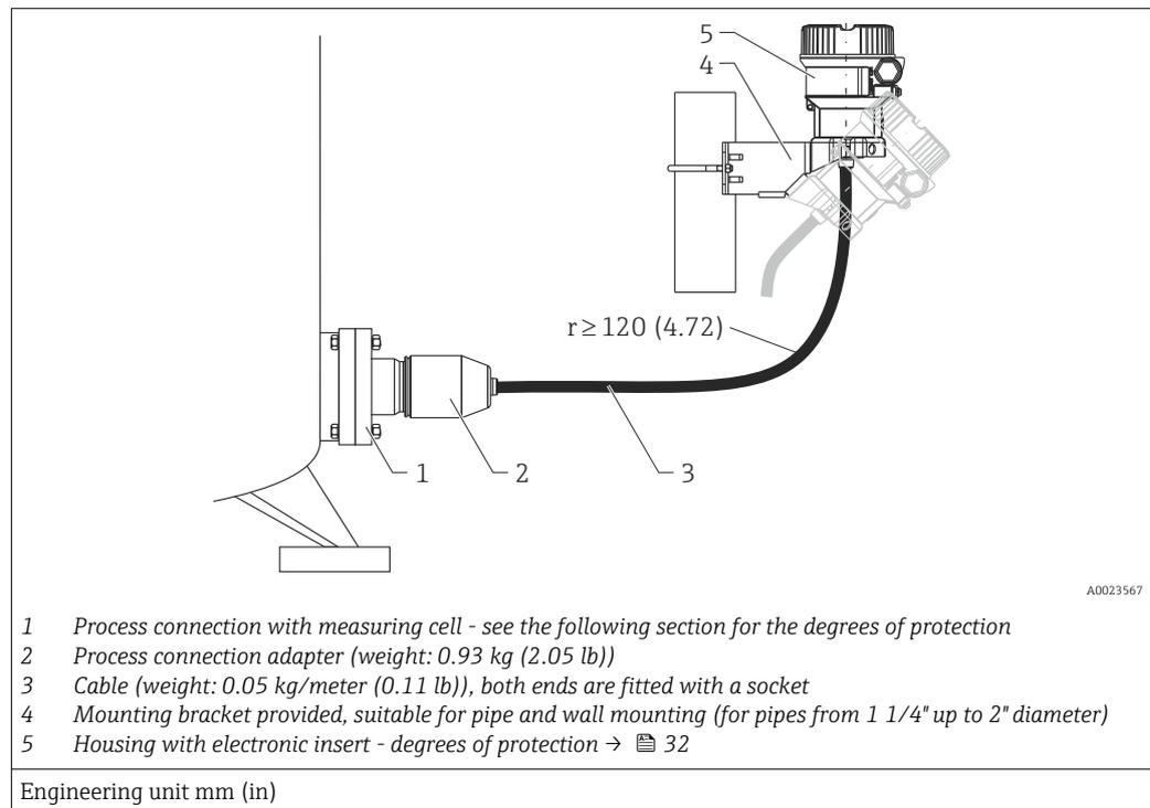
Degree of protection for the process connection and measuring cell with the use of
