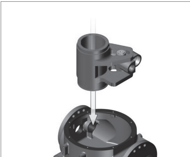
Step 5. Install the yoke assembly in the bottom bearing (56) of actuator with bottom side O-ring seal (36).
