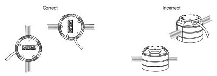
The pipe must be filled with liquid and free from air bubbles. Avoid air purge of the system which would cause damages and to prevent damage from dirt or foreign matter, we strongly recommend the installation of a 75  $\mu$ m strainer as close as possible to the inlet side of the meter.
