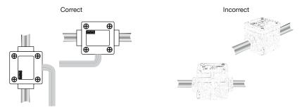
The pipe must be filled with liquid and free from air bubbles. Avoid air purge of the system which would cause damages and to prevent damage from dirt or foreign matter, we strongly recommend the installation of a 75 µm strainer as close as possible to the inlet side of the meter.
