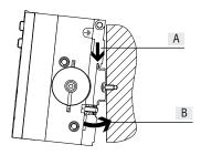
The MPA-L valve terminal is screwed onto the mounting surface using four M4 and two M6 screws or using six M6 screws. The mounting holes are on the left-hand and right-hand end plate and on the pneumatic interface. Optional mounting brackets are also available.
