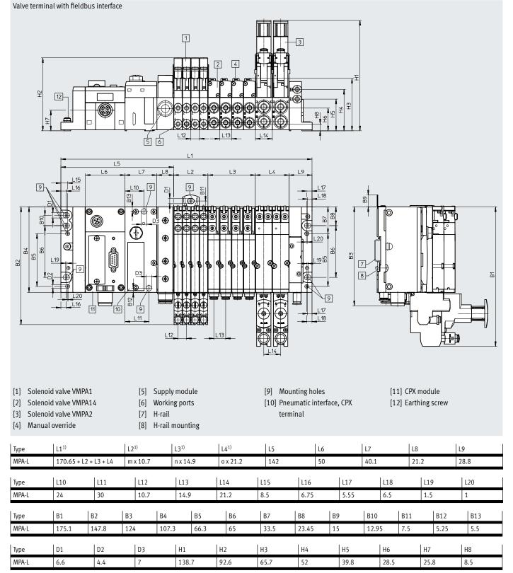
1) m, n, o = number of sub-bases/valve positions (m = width 10 mm, n = width 14 mm, o = width 20 mm)
