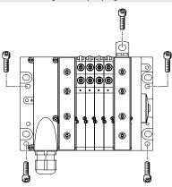
Wall mounting - Fieldbus interface (CPX terminal)
