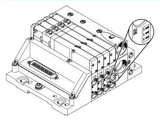
MPA-L offers a number of options for creating pressure zones if different working pressures are required. A total of up to 20 pressure zones can be created.
