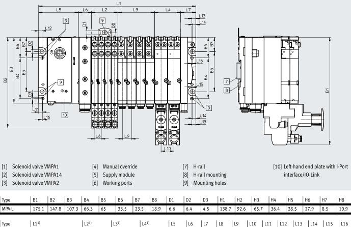
1) m, n, o = number of sub-bases/valve positions (m = width 10 mm, n = width 14 mm, o = width 20 mm)
