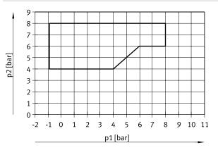
For valves in width 10 mm with code for position function 1-32: MU, NU, KU, HU
