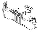
An adjustable pressure regulator can be installed between the base plate and the valve to control the force of the actuator. This pressure regulator maintains a constant output pressure (secondary side) independent of pressure fluctuations (primary side) and air consumption. Standard version:
