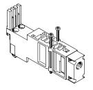
This vertical pressure supply plate enables an individual valve to be supplied with individual operating pressure independently of the operating pressure of the valve terminal. The exhaust and pilot air supply of the valve are still provided via the central ports of the valve terminal.
