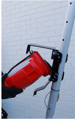
Fig. 8 Insert FABX2R or FABXLR into the bracket as shown seating the cable end in the bracket
