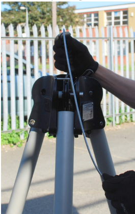
Fig. 4 Pull cable up to tripod head and insert hook through central hole.
