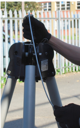
Fig. 10 Pull cable up to tripod head and insert hook through central hole.
