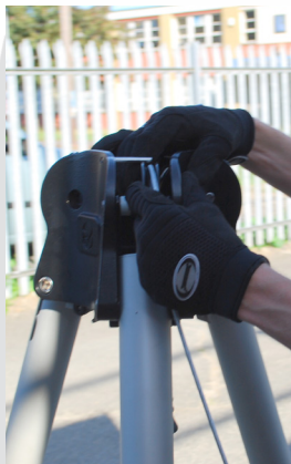
Fig. 11 Slide spring loaded pulley to right, insert cable in pulley groove, and release pulley.
