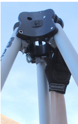
Fig. 4 Open legs out and ensure sprung loaded tabs lock out in position.
