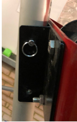
Fig. 2 Align the holes in the bracket with the holes in the tripod leg and insert a detent pin.
