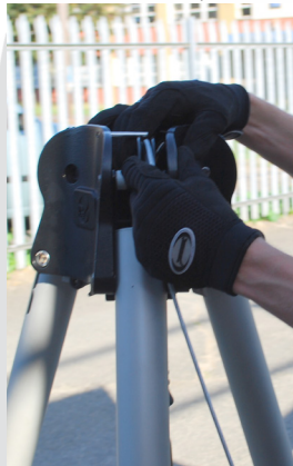
Fig. 5 Slide sprung loaded pulley to right, insert cable in pulley groove, and release pulley.
