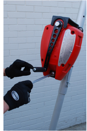
Fig. 9 Secure with M12 bolt.
