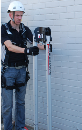
Fig. 1 Unpack tripod and stand upright.
