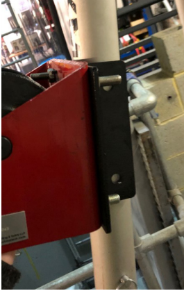
Fig. 1 Slide the bracket (WG-02) which is fixed to the winch onto the tripod leg.
