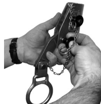
Figure 10 – Connect to Lifeline: Step 4
