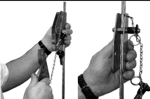
Figure 9 – Connect to Lifeline: Step 3
