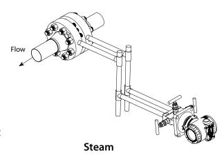
Note: For steam or other elevated temperature services, it is important that temperatures at the process connection do not exceed the transmitters process temperature limits.
