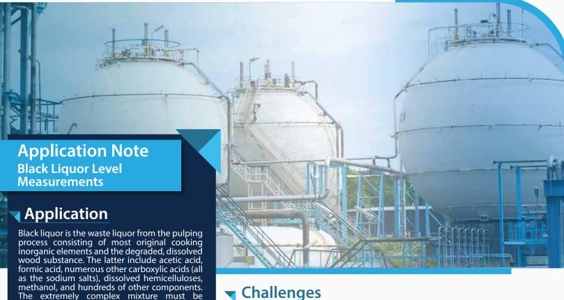
Black liquor offers some unique measurement challenges, such as it is an extremely alkaline material that varies in density, depending on upstream flow. It must undergo many processing stages before the cooking liquor is regained. Containment of the spent liquor must be measured and controlled in a series of intermediate storage tanks. To add to the challenge, the black Liquor is sticky and easily coats the surface.
